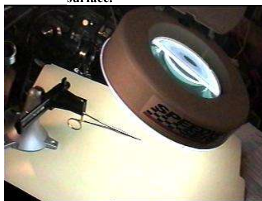
A lighted magnifier is an absolute must! Under it is the Author's Panivise Jr. holding the hemostat holding a tiny chip to be tinned.
